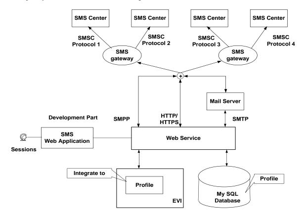
Figure 2: SMS Spot Application Architecture
