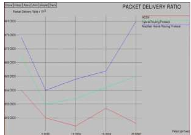
Figure8. The packet Delivery ratio comparison among the three routing protocols for 100 nodes of the network
