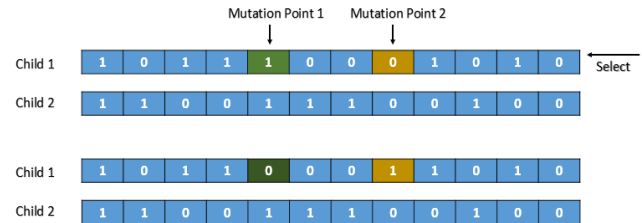
Figure. 3 Bit change mutation operator suggested
