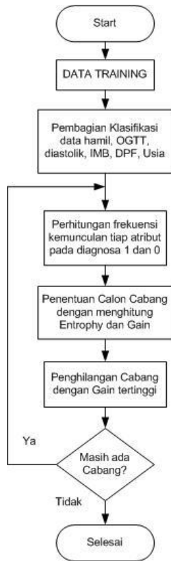
Figure 3. Flowchart of C4.5 Algorithm
