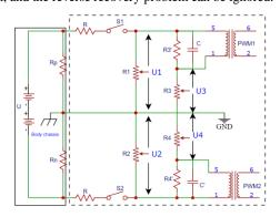
Fig. 3 Schematic diagram of voltage injection insulation detection
