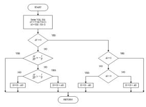
Figure 4. Flowchart Incremental Conductance
