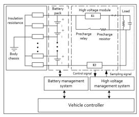
Figure. 1 Vehicle chassis insulation electrical system
