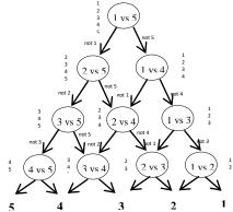
Figure 3. Illustration of DAGSVM for the 5 class classification
