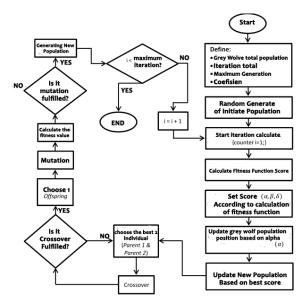
Figure 7. Hybrid Grey Wolfs Optimization – Genetic Algorithm (HGWGA) Flow Method Diagram
