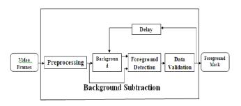
Figure. 3 Background Subtraction Flow Chart
