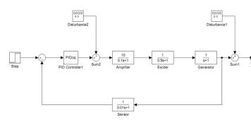
Figure 8. The diagram block of the automatic voltage regulator (AVR) loading test
