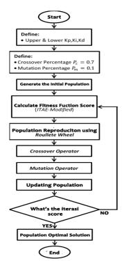
Figure 4.4 Genetic Algorithm (GA) Flow Method Diagram
