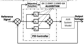
Figure 4. PID-based AVR system diagram block using the installation of Artificial Intelligent (AI) method
