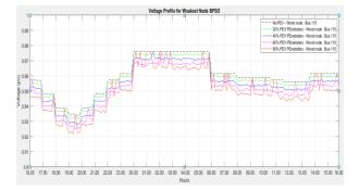
Figure 8. Voltage profile for the weakest node using BPSO algorithm
