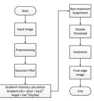
Figure 2. Canny edge detection feature extraction flowchart
