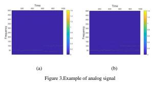
After that, 282 signals was intercepted from the actual seismic data, each signal had 1501 sampling points, and the sampling frequency was 2ms. We selected one of the signals for analysis. From its time domain image, we could see that the signal burr was significantly reduced after denoising, and then from the frequency comparison diagram, we could see that the high-frequency noise was effectively removed, and the original characteristics of the signal were not greatly affected.
