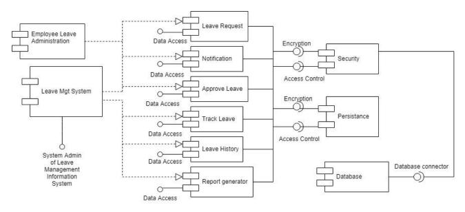
Figure 10. Screenshot of the Component diagram of the System
