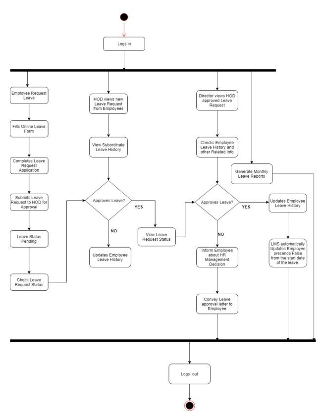
Figure 6. Activity diagram for the Leave Management System
