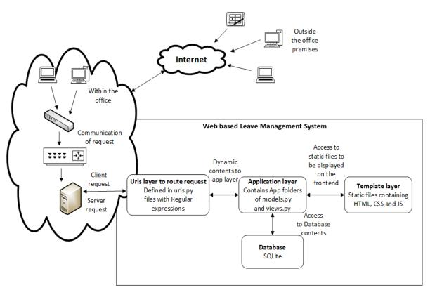
Figure 4: System Architecture for the Leave Management System
