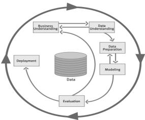
Figure 1: Cross Industry Standard Process for Data
