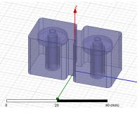
Fig. 5 resonator coupling model
