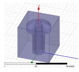
Fig. 2 Single-cavity filter model
