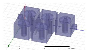
Fig. 6 The established fifth-order filter resonance model.
