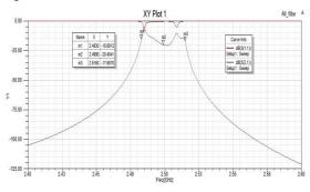
Fig. 7 Initial simulation results of integral filter
