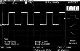
Figure 8. Example of 50% PWM waveform and 50 kHz frequency
