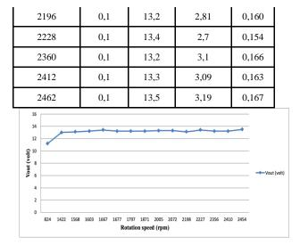
Figure 14. Graph of output voltage versus rotation speed
