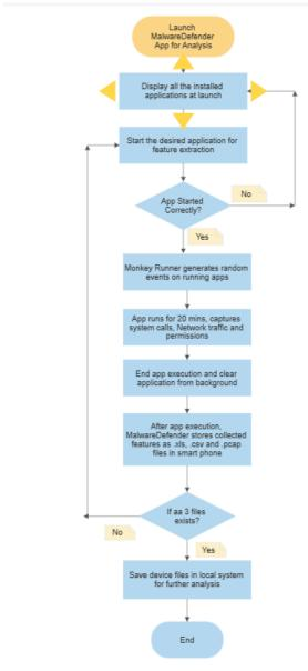
Figure 3 MalwareDefender – Architectural Flow of Dynamic Analysis Tool
