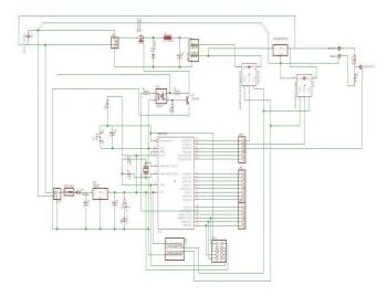
Figure 5. Overall circuit of the charge controller system
