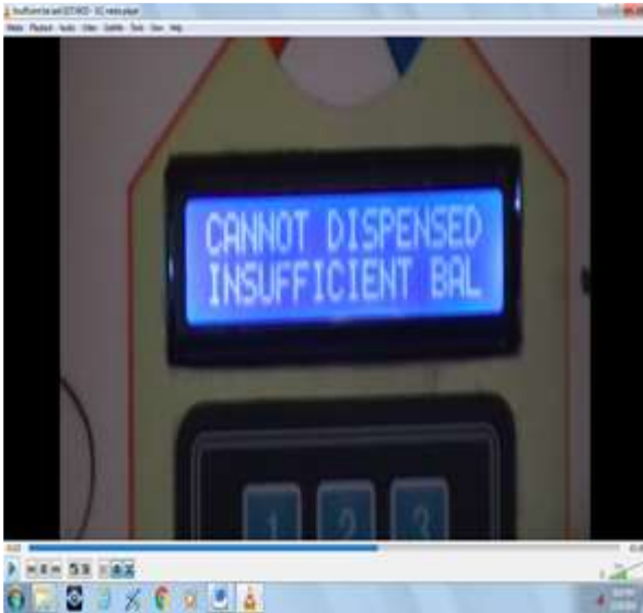
Figure 14: Message displayed if the card has insufficient balance
