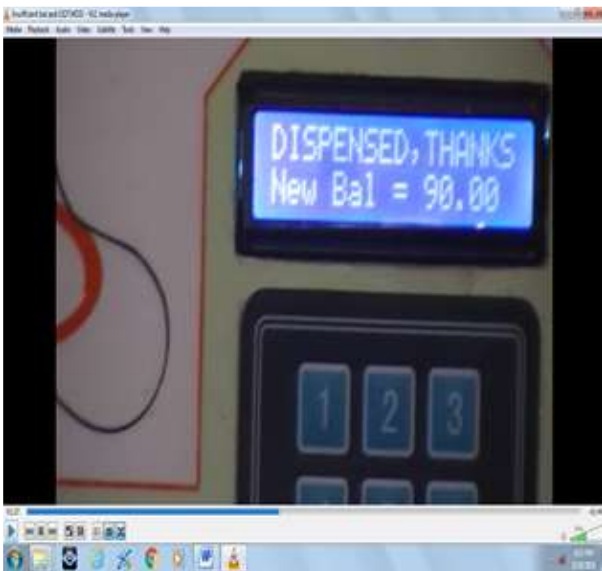
Figure 10: The vending machine displaying the balance after the transaction
