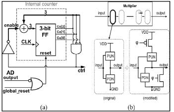
Figure. 2(a) Schematic of *ctrl* signal generator. Internal counter sets *ctrl* signal to "1" when all input samples inside MCSD are smaller than *xth* (m=4 case).(b) Modified gate schematic to turn off multiplier.
