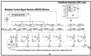
Figure. 3 Proposed FIR filter with fixed co-efficient
