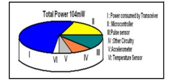
Figure 10. Power consumption in each subcomponent
