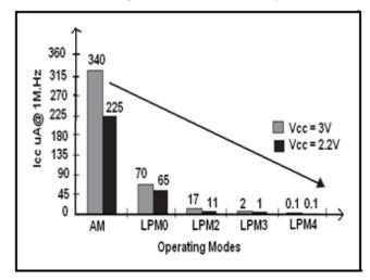
Figure 1. Graph showing the current consumption in different operating modes of MSP430 family.
