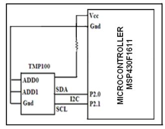
Figure 4. Interfacing of Digital temperature sensor TMP100
