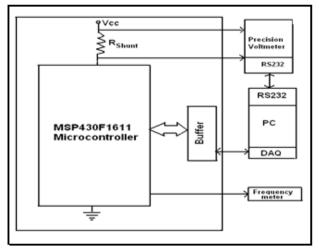
Figure 8. Measurement of current consumption
