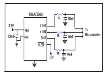
Figure 6.Accelerometer Circuit for respiration measurement
