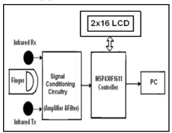
Figure 5. Block diagram of Pulse rate measurement
