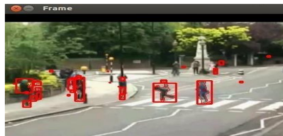
Fig. 10. Height-width based approach contains only pedestrian
