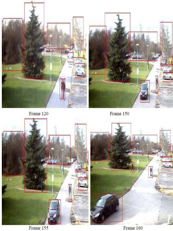
Fig. 6. Static and dynamic object detection from PETS dataset
