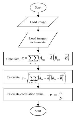
Figure 8. Calculating correlation stage flow chart
