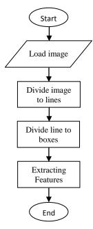
Figure 8. Segmentation stage flow chart
