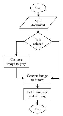
Figure 4. Preprocessing stage flow chart
