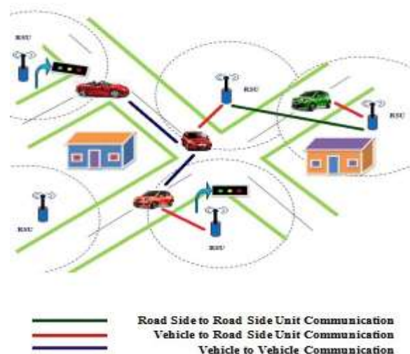
Fig. 2: Vehicular network architecture
