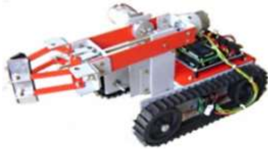
Figure.2 Robotic rover with gripper arm
