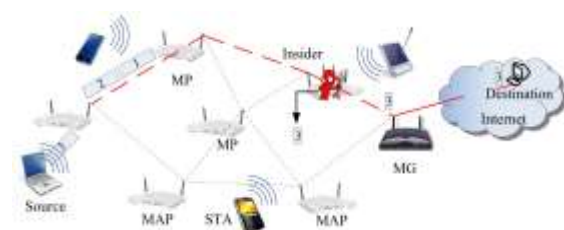
Fig. 4. An insider selectively drops cumulative TCP acknowledgments and forces end-to-end data retransmissions.
