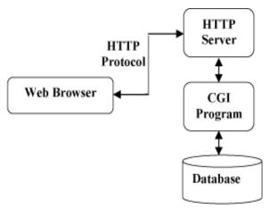
Figure 4. The HTTP Protocol in Communication Model
