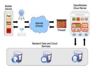
Figure.6. The open mobster architecture [12]
