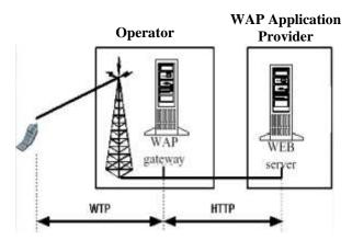
Figure 1. Gateway equipment in the operator premises
