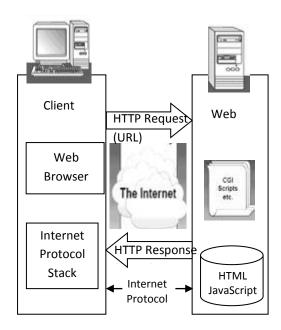
Figure 5. A HTTP Client-Server Request-Response Architecture
