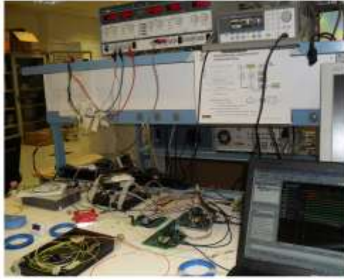
Figure 1.2. Experimental Setup to Acquire Coded Stokes and Anti-Stokes Traces
