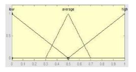
Figure. 1 Diagram of membership function of priority parameter
