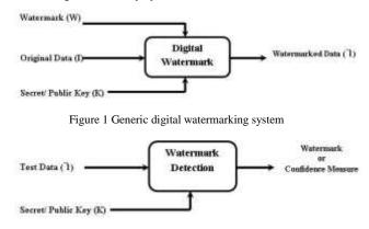
Figure 2 Generic digital watermark recovery system
