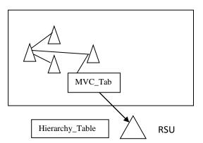
Figure 9. MVC\_Table submission and Hierarchy\_Table formation at RSU
