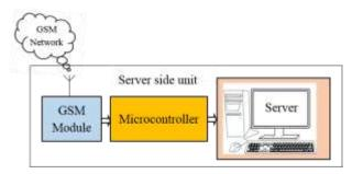
Figure. 5 The functional diagram of the server side unit.
