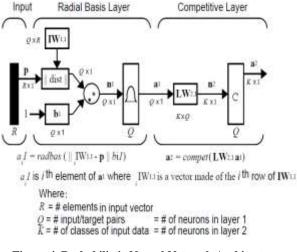
Figure 4. Probabilistic Neural Network Architecture.
