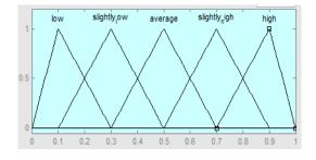
Figure. 4 . Diagram of membership function Response Time
