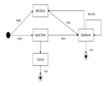
Figure 5. Statechart diagram of input and edit data
