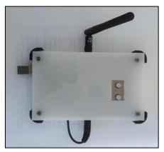
Figure 9. The Receiver of Obstacle Height Monitoring System
