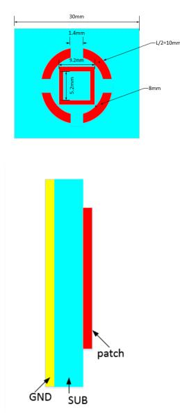
Figure.9 Antenna structure
