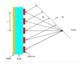
Figure.1 Reflective array antenna working diagram
