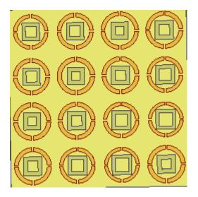
Figure.14 Microstrip reflective array antenna
