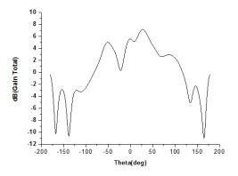
Figure.14 Gain curve of the reflective array
