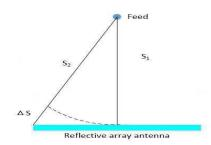
Figure.2 Spatial wave path difference between the units of the reflective array antenna
