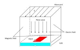
Figure.4 Waveguide simulator model
