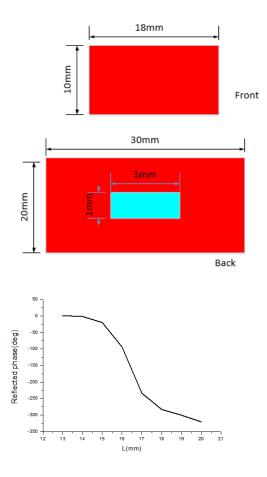
Figure.8 Antenna model and its phase shift range
