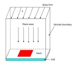
Figure.3 Infinite period model
