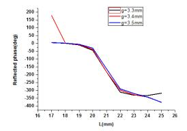
Figure.12 Effect of different parameters g on phase shifting performance
