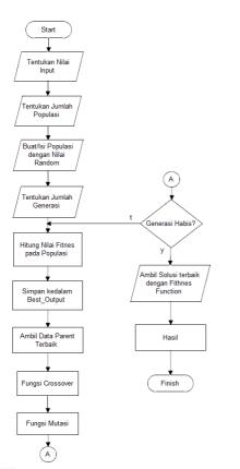
Figure 4. Flowchart of the Genetic Algorithm (GA) Method
