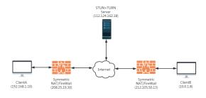
Figure.4 Symmetric NAT / firewall network topology
