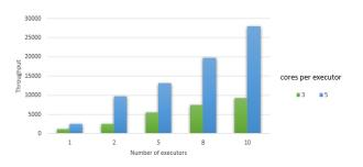
Figure 8: Throughput when changing the executor's number and number of cores at each executor for the proposed architecture
