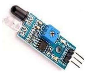
Figure 1 Infrared transceiver module.
