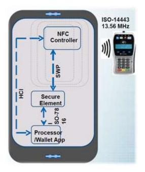
Figure 2.2. A mobile phone with a Secure Element. (*Image Source; Swaminathan, 2017*)
